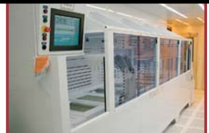
Automated wet bench with new IDX controls
